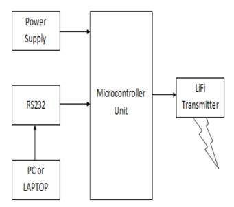
Fig.3 Block Diagram – Transmitter Unit
