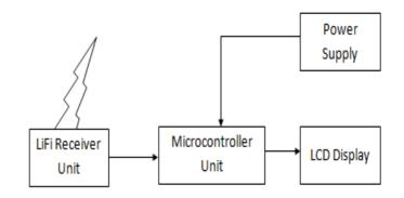
Fig.4 Block Diagram - Receiver Unit
