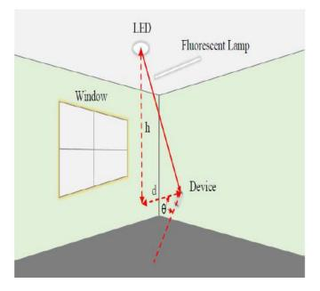
Fig.1 Indoor visible light communication system
