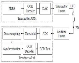
Fig. 2. Block diagram of a VLC system.
