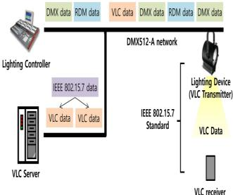
Fig.5 VLC Data Transmission on DMX512-A Network
